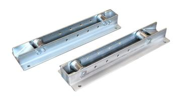
D-496-01 Roll on Drum Stand allows a range of drums to be accommodated to suit the majority of applications. Manufactured in steel, with ball bearings in the rollers, the stand is suitable for pulling off cable from the drum.
