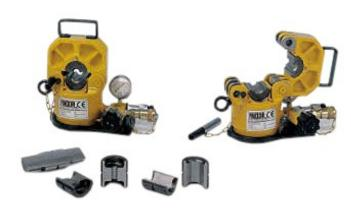
The hydraulic Press of 55 tons compressive capacity is suitable for compression of joints on conductors and steel ropes on medium and high voltage power transmission lines. The unit features excellent weight/power ratio (2.9 ton/kg) and is easy to operate on suspension working platforms and steel towers thanks to the specific cover fitted on the press body. Maximum hexagonal key of 44 mm allows pressing of a conductor of 31.5 mm diameter.
