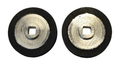
These drive wheels have parallel (un-grooved) surfaces and are made of a softer material than standard, C1300-DW- 90 drive wheels. Recommended for use with small cables 1mm to 2.5mm, or when extra grip is required.
