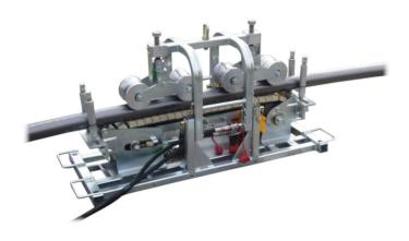
The C-1350 Cable Pusher has been designed to assist the laying of electrical cables or cylindrical elements. The unit has a profiled drive system to grip the cable, with a load applicator of adjustable upper rollers.
