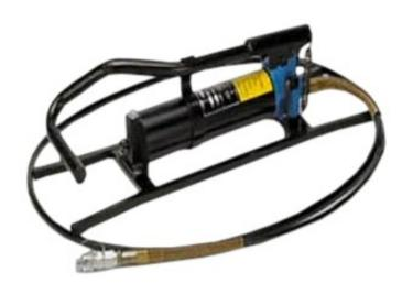
Foot operated double speed pump, developing a maximum pressure of 700 bar. The pump is supplied with 3m long high-pressure flexible hose complete with female self-lock quick coupler. Pressure can be withdrawn at any time during operation by depressing the release lever. A solid shaped stand gives the pump stability during operation.
