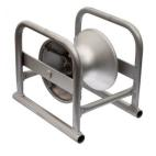
A cable roller designed to bridge existing cables. Fitted with oil-impregnated bearings for use in adverse site conditions. Tubular steel frame construction, choice of two types of rollers.
