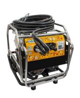
This unit is powered by air-cooled, 8hp petrol driven engine, delivering 20 litres/min at a working pressure of 138 bar from the hydraulic circuit. The circuit is protected with return line and suction filters. CE approved.
