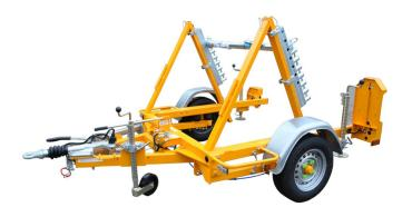
The C-751 Drum Trailer comes in three versions, and provides a compact and secure method of drum transportation. Manufactured in strong steel sections, it incorporates manually operated hydraulic lifting of drums.
