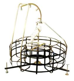
The Micro Cable Fleeting device has been developed to enable longer lengths of fibre optic cable to be laid from a single drum. Employed when the cable needs to be removed from the cable drum, in preparation for blowing the second section.
