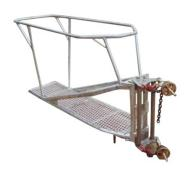
Manufactured in tubular aluminium, incorporating a non-slip open plate platform. Platforms have a safe working load of 250kg. All models feature a serrated pole gripping device and are lightweight and simple to apply.
