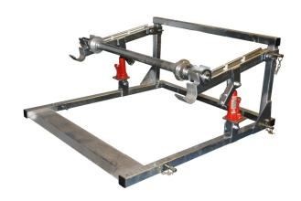
Designed in sections for ease of transportation and simply slots together to form a rigid and stable drum stand. The shaft is fitted with bearings and drum location collars are also included. Two hydraulic jacks provide drum lifting.
