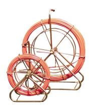
A high quality fibreglass rod, specially constructed to provide exceptionally high tensile strengths, whilst retaining flexibility. The 80% fill rate glass fibre core is reinforced with a high strength resin. A braided reinforcing wrap is added before the final polypropylene wear resistant protective coating is applied. The continuous rods range from 4.5mm – 14mm with lengths from 30 metres – 300 metres.
