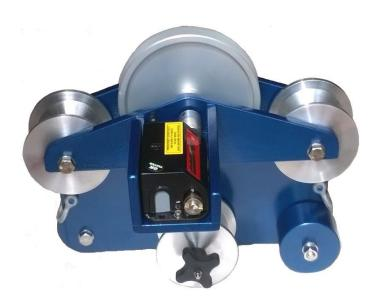
This machine has been designed to measure lengths of overhead cables. The unit is hung on the cable and a vertically movable pulley is used to clamp the measuring wheel to the cable. A shackle is provided to enable the machine to be pulled along. A mechanical counter then displays the length/distance that the machine has moved. Its primary use is for positioning of spacers on overhead power lines. Can accommodate cable sizes between 8-43mm diameters.
