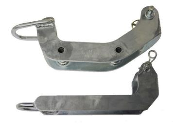
Special purpose device designed to meet Electricity Board Standards. Fits at the end of an insulator set when sagging and is used for making off dead ends on wood pole lines.
