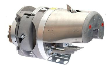
Our compact Model C2 Cable Lasher is perfect for lashing smaller diameter aerial cables to supporting strand with stainless steel lashing wire. The new design improvements make the C2 equally suited for new construction or overlashing up to its full  $1^{7}/8$ " (46 mm) bundle capacity.
