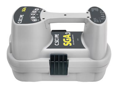
Enhance the detectability of cables and pipes; trace out the route of specific services. Use the signal generator to transmit an easily identifiable signal along a cable or pipe. Trace the lines using the Cable Avoidance Tool. New industry accepted 33 kHz operating frequency for clearer signal reception.
