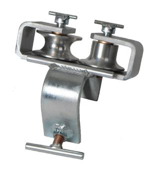
Designed to mount onto angle cross arms up to 100mm. Sheaves are fitted with sleeve bearings. This design allows conductors to be strung around route deviations.
