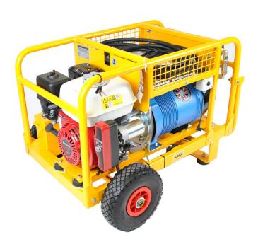
A compact 10 Bar compressor specifically for use with the CBS C-1800 Accelair2 Blown Fibre Unit. The compressor is fitted with aftercooling, filtration and air drying essential in providing the optimum viscous drag effect for maximum fibre blowing length.
