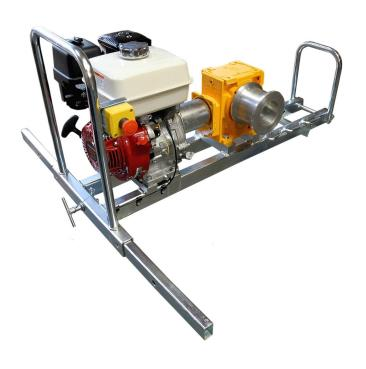
The C-1035 Lightweight Capstan Winch is designed for use over manholes. Powered by a 5.5HP Honda engine through a right angle gearbox, the C-1035-05 offers a pulling capacity of 500kg with a lighter weight design than the 1000kg version.
