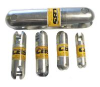
Swivels are essential for effective pulling operations of underground cables and overhead conductors. The swivels are fitted with bearings to prevent build up of twist in the cable pulling bond. CBS swivels are precision manufactured in high-grade steel with a plated finish.
