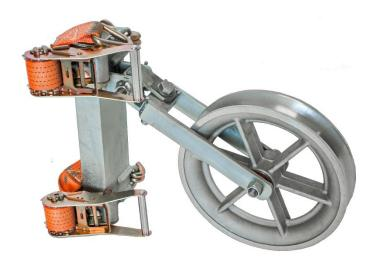
The block allows the stringing operation to be fed up or down poles, when access at the rear of the pole is not available. 300mm sheave with quick acting ratchet fixing and a conductor side gate.
