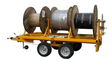
A uniquely versatile tool. A single operator can independently control the tension of all three conductors.
