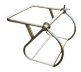
The Drum Cradle has been designed to lift  $2 \times 1200 \text{ mm}$  maximum diameter of micro duct with a total weight of 200kg. The Drum Cradle is a rigid tubular steel construction with a detachable drum spindle and drum spacer, the drum spacer prevents the drums from rotating against each other.
