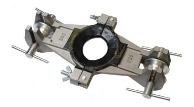
Suitable for 33kV insulator, has two sheaves for stringing, which are lowered for making off onto insulator. The D-733 is designed to fit insulators from 115-135mm, whilst the D-917 is designed to fit insulators from 70-90mm.
