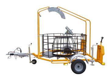
The Fleeter replaces the manual method of "figure of eighting" cable and provides protection and security for the cable. Following installation of the cable in the first leg of the duct route, the balance of the cable is removed from the drum and fed into the Fleeter, thereby releasing the cable end ready for blowing into the second leg.
