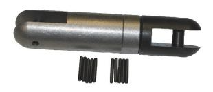
Fused swivels are used in applications where the pulling force must not be exceeded. The fuses are replaceable and allow the swivel to break when the maximum applied load equals the rating of the fuse.
