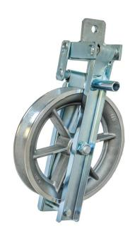
Capable of accommodating the larger conductor, this aluminium suspension block has an automatic safety gate and steel frames. Hole mounted to fit insulator clevis.
