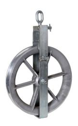
Single sheave aluminium suspension block with spring loaded safety gate & steel zinc plated side frames. D-700 has a swivel oval eye arrangement. D-702 has a hole mounting to fit insulated clevis.
