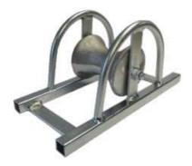
Designed for use in narrow trenches. Lightweight assembly suitable for cables up to 76mm dia. Zinc plated steel frame fitted with large waisted solid aluminium roller running on low friction sintered bushes.
