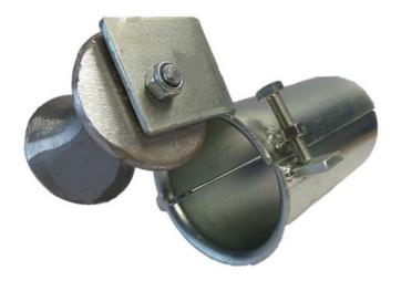
In separable hinger halves to guide the cable through the duct to avoid damage to both the cable or the duct. Fitted with a guide roller for additional rope guidance and protection. Zinc plated finish.
