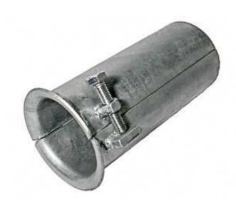
Manufactured from Zinc plated Steel, the Bellmouth comes in separable halves to guide the Cable through the Duct to avoid damage to both the Cable and Duct. Also available with rollers.
