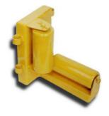
Purpose designed for taking the heaviest cables round difficult corners and bends. Incorporates a vertical and horizontal roller 75mm diameter on low friction sintered bushes
